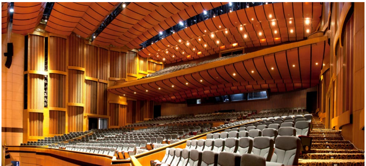
Figure 10: 1100 seat multipurpose theatre with adjustable 3-sided rotating wall reflective/absorptive/dispersive panels.
